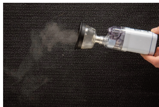
Figure 4 A plume of nebulized aerosol being generated by a handheld, battery-powered nebulizer. The device would be attached to a face mask for drug delivery to a cat
